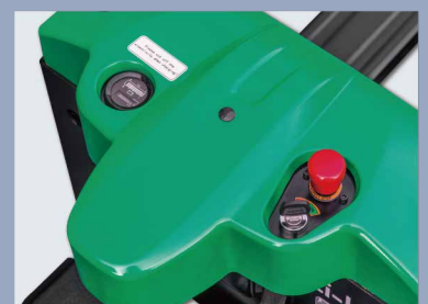
The key switch, emergency cut off switch, and battery meter are all easily accessible by the operator.
